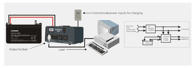
Wiring for bus cut-in (only suitable for machines whose power is equal to or over 2kVA)
